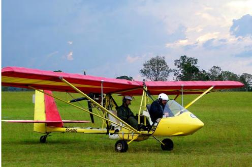
Under Peter's guidance, taxiing was a breeze so long as the speed was kept low because the brakes were not especially efficient. Although the rudder was effective in the slipstream, the tail-wheel springs were soft and the tailwheel was less useful for steering than I expected. The runup was uneventful and the pre-take-off checks uncomplicated – this is a very basic aeroplane. With checks completed, a lookout showed that there was no other traffic and the runway was ours. We were ready to go.
