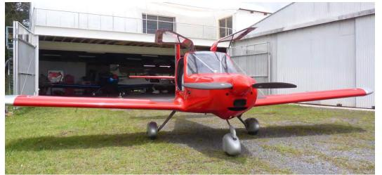
As I suspected, the stall at 40 kts indicated was a non-event except for the high nose attitude – another attribute of low aspect ratio wings. Again, the side stick was easy to use and fingertip light. Regardless of the aeroplane configuration, each stall was preceded by a deepening buffet and then a gently nose sag with little or no tendency for a wing to fall away. Instant recovery came with appropriate forward stick, and the IAS rose quickly.
